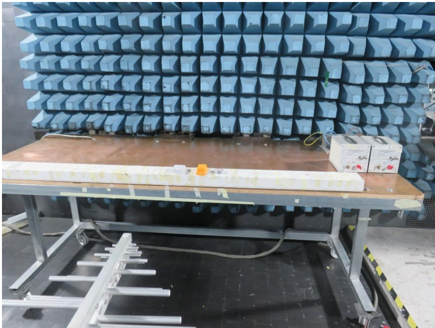
Photograph 4.2: RE Antenna positioning, Horn antenna, 200MHz – 1GHz
